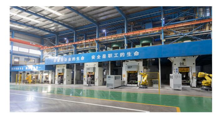
Our forming workshop is equipped with multiple automatic hydraulic presses, ensuring precise compaction of high-density refractory bricks.
