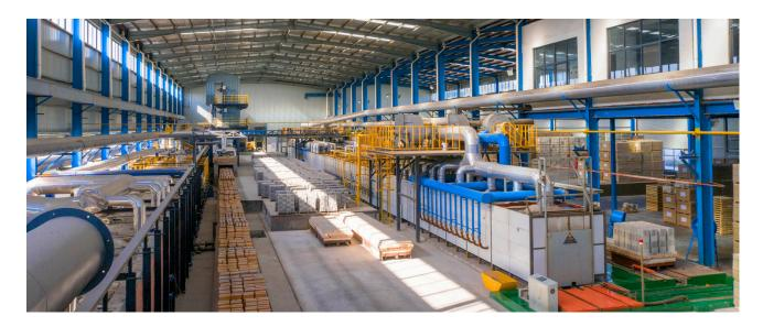
The tunnel kiln firing workshop uses an advanced control system to ensure stable high-temperature sintering of refractory bricks. The process delivers consistent quality, excellent volume stability, and reliable thermal performance.
